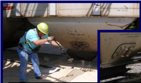
Pulling / Pushing Using a bar to manually open or close a rail car hopper
