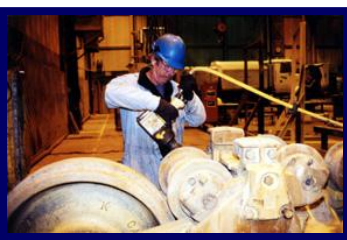
Hand Arm Vibration – operating a pneumatic wrench
