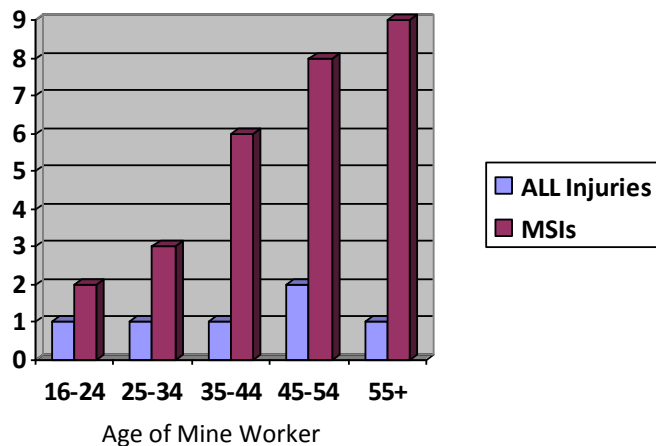
Median days lost for musculoskeletal injuries relative to all injuries/illnesses (MSHA Injury Data, 1992-2002). (1)
